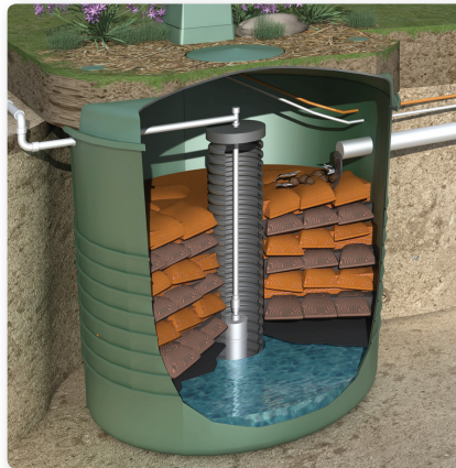
Cross-section of a Biolytix System
